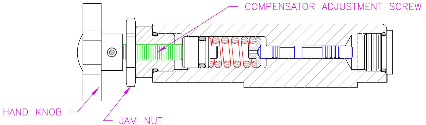
1. HOLDING TIGHT THE HAND KNOB, UNLOCK THE JAM NUT
